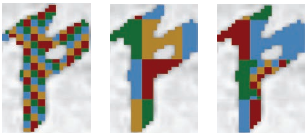
Fig. 6 The tessellation of the letter ‘p’ at two different granularity levels. From left to right the squares have a lateral length of 2, 11, and intermixed, 2 and 11 pixels.
